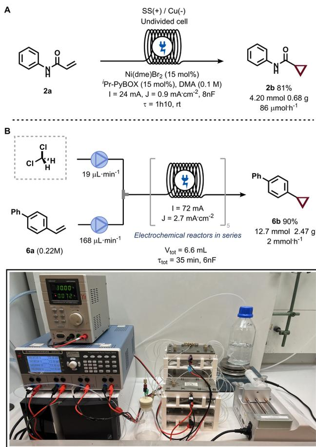
**Scheme 4.** Scaling up the electroreductive nickel-catalyzed cyclopropanation of alkenes. **A.** Productivity assessment of the reactor over 49 hours. **B.** Multi-gram scale electroreductive cyclopropanation in continuous flow with 5 reactors in series which are powered in parallel.
